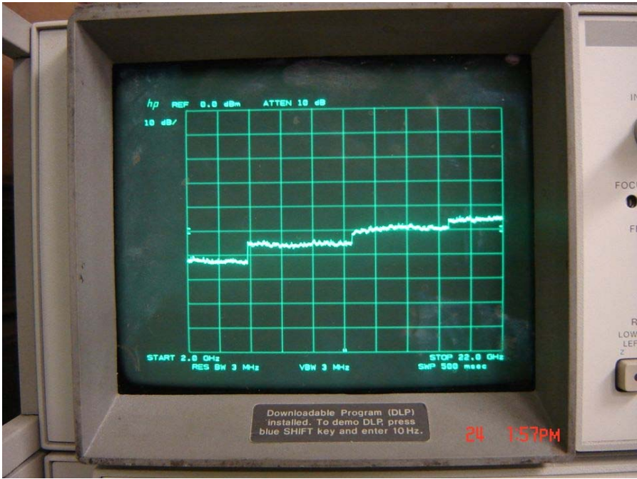
Figure 6. 2-22GHz w/ inputs shorted.
