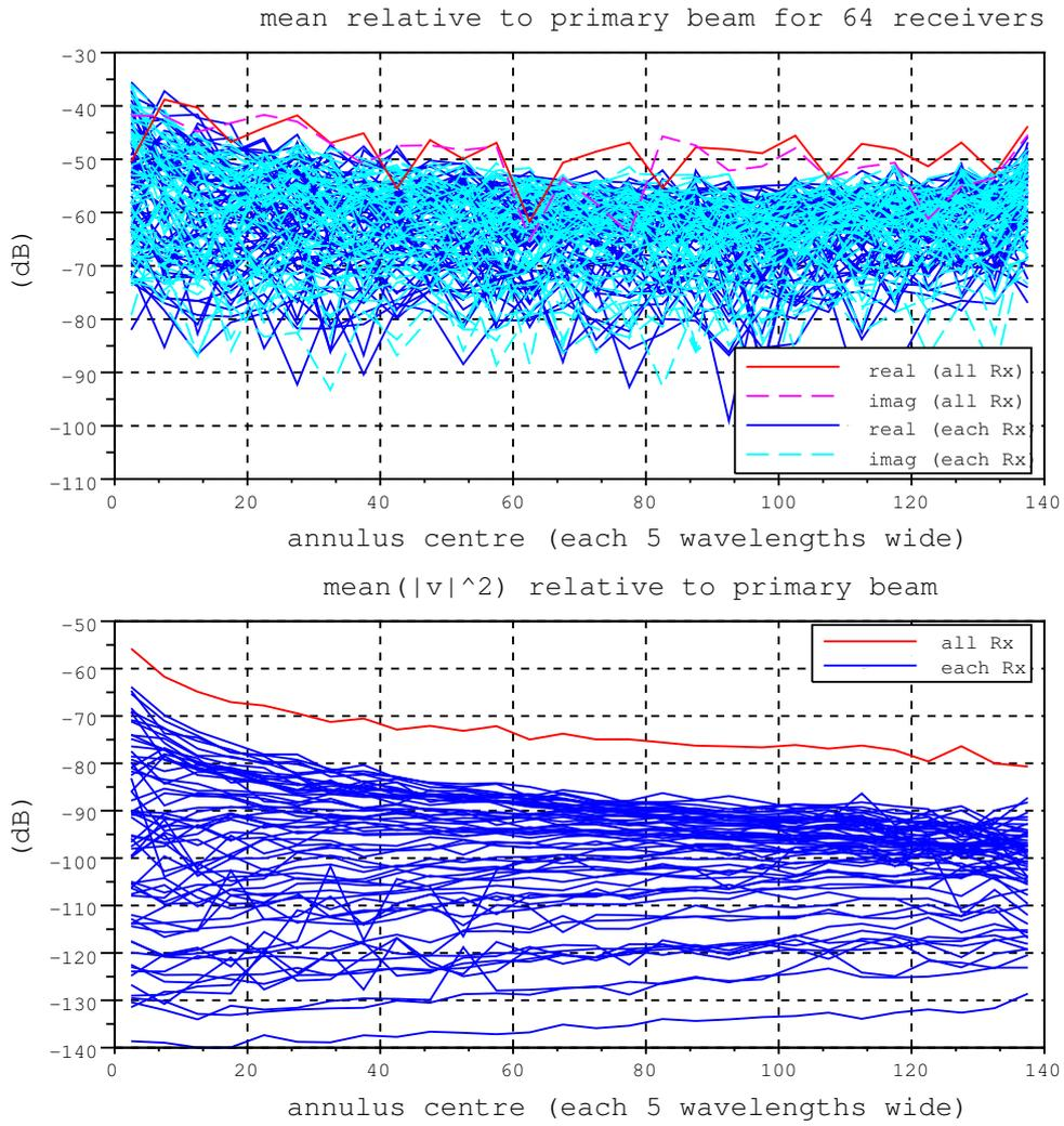
Figure 1: Receiver RFI relative to the incident RFI level. RFI phases and the attenuation due to path-loss were calculated for each visibility, but the sidelobe gain of the antennas has not been included. This is for a single snapshot.
